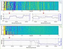
Lab test for geoelectrical monitoring of earthen levees
